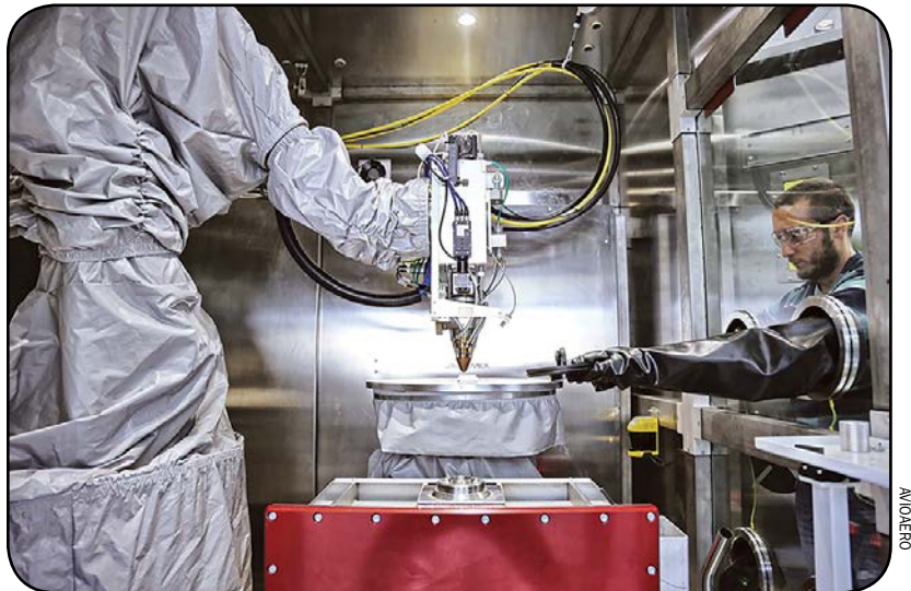
Avio Aero is hoping to replace legacy repair techniques with cold spray.
