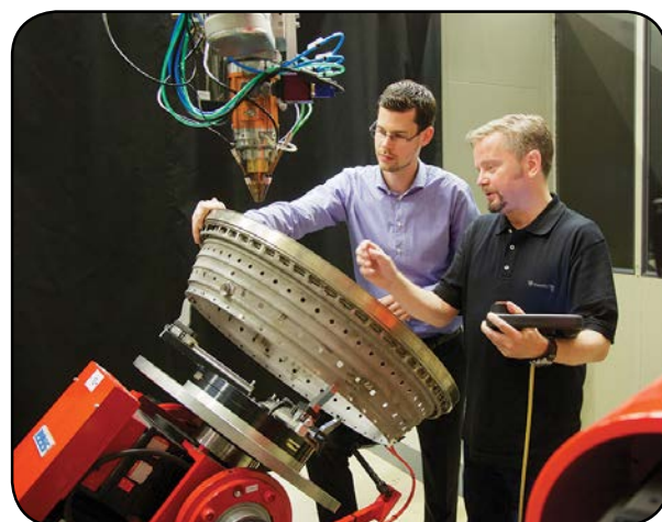
Lufthansa Technik’s automated repair robot tests for combustor cracks.
