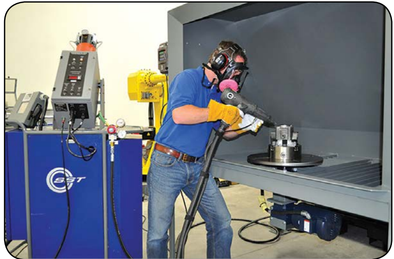
A technician uses a hand-held cold-spray system.
